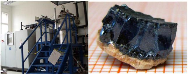
Fig. 1: Skull-melter at TU Berlin (left) together with CeO<sub>2-5</sub> single crystals (right).
